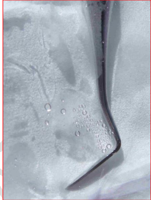
Figure 4.8 Condensation within an instrument pack
